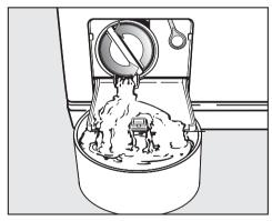
■ Slowly and carefully unscrew the drain filter to let the water out.
